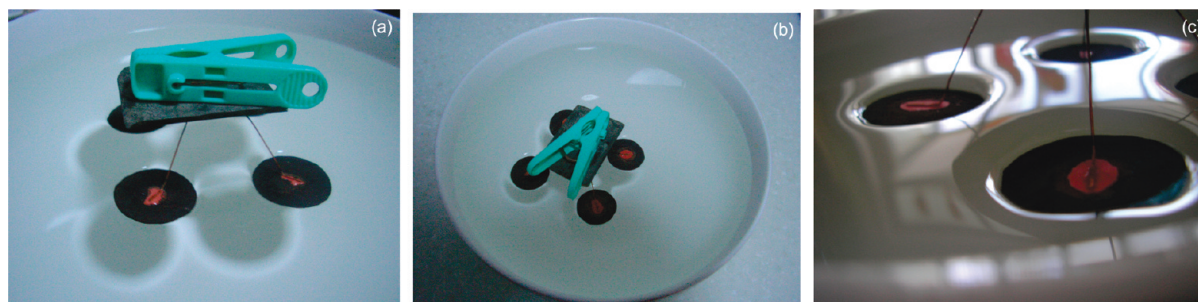
FIGURE 1. Water strider-like model carrying a 5.0 g plastic clap floating on the water surface: (a) side view of the model, (b) top view of the model, (c) dimples around the “legs” of the model. The net weight of the model is 1.1 g, and each “leg” has a diameter of 2.0 cm. The copper foils used in the model had a contact angle of 155.4°.
